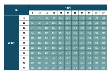
BRD Bare Shaft Damper Weight Matrix - 250D
